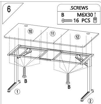
Avoid excessive tightening screws before all the screws have all screws are screwed into the screw holes correctly.
